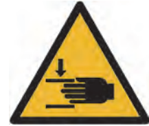
Warning, Crushing of Hands
