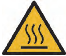
Warning, Hot Surface
